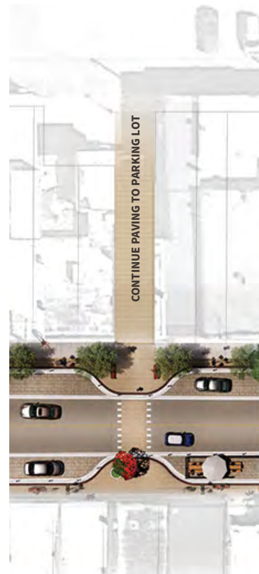
Typical crosswalk with continuing paving to parking lot
