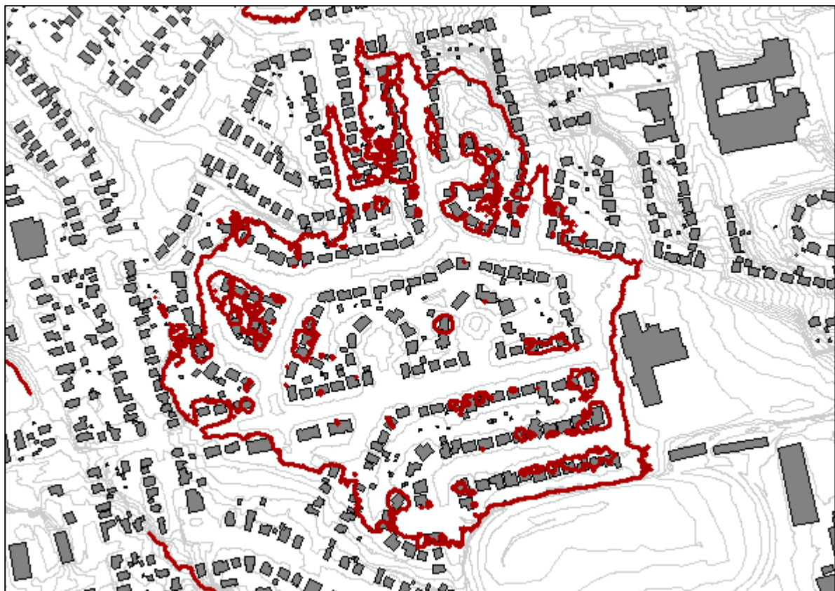
Figure 3-3: Area Subject to Potential Basement Flooding Risk from Foundation Drain or Private Drain Connections to Storm Sewers (HGL within 1.8 m of the ground, 2-year storm)
