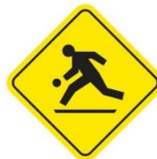
Wc-3 (Playground Area)
